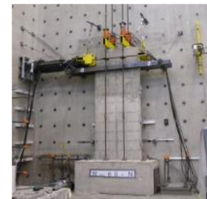
Wall with lap splices of length of 60 bar diameters and unconfined boundary elements
